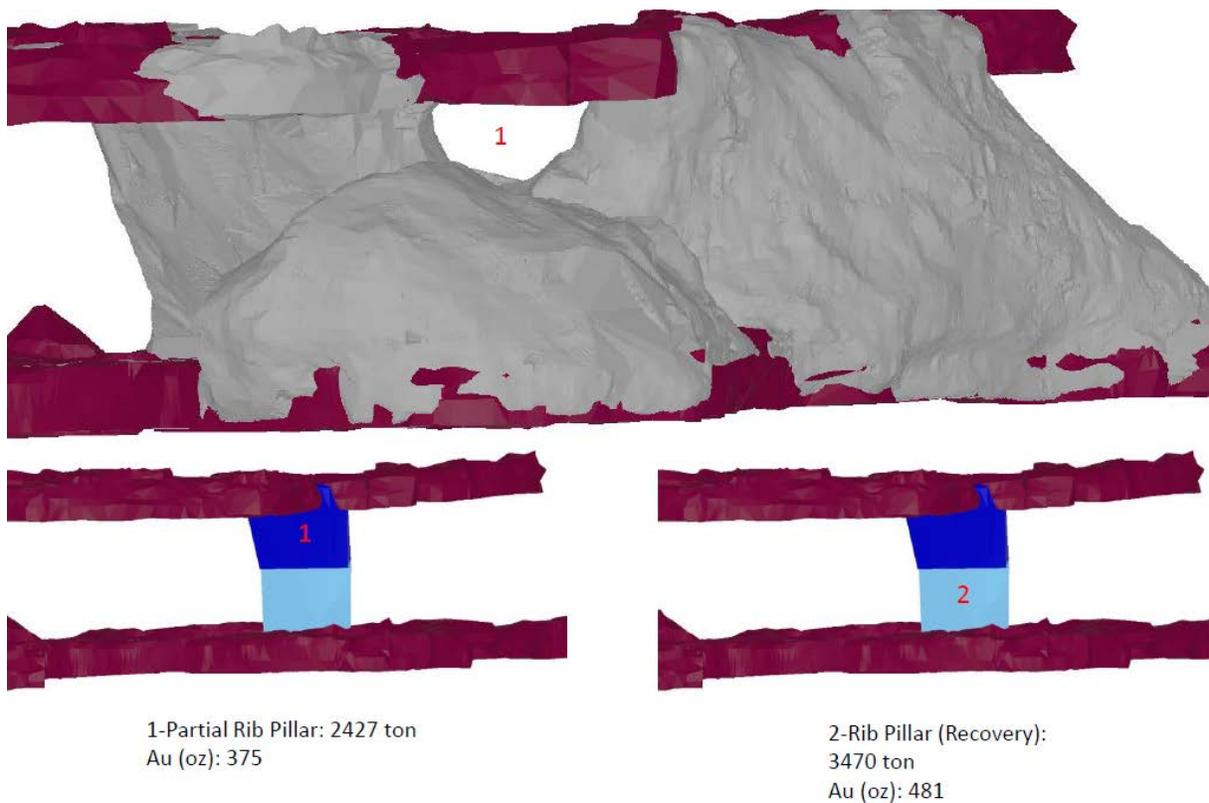
In order to reduce external dilution, stope pillars (1) are added in low grade areas as shown in Figure 15-2. A rib pillar is initially planned between the two stopes. Once the stope on the left is mined, the lower portion (2) of the rib pillar is recovered by drilling from the lower drill horizon, and then the next stope is mined
