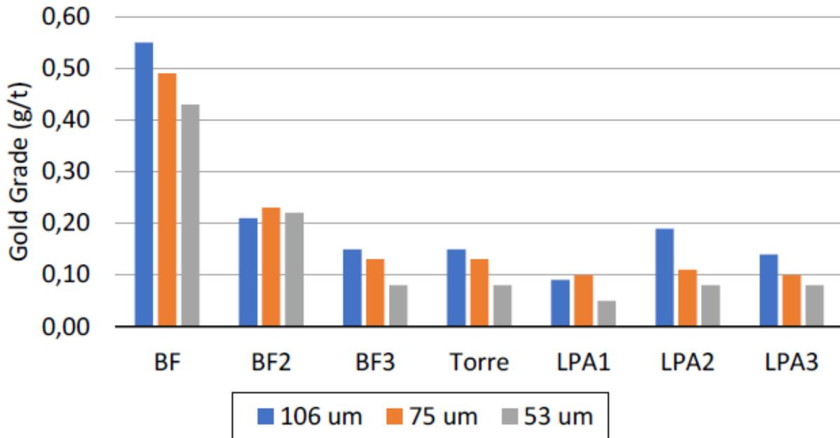
The results show that a finer grind ( $P_{80} = 53 \mu\text{m}$ ) reduces the values of gold content in tailings in flotation tests with consequent increase in overall recovery (gravimetric concentration + flotation).
