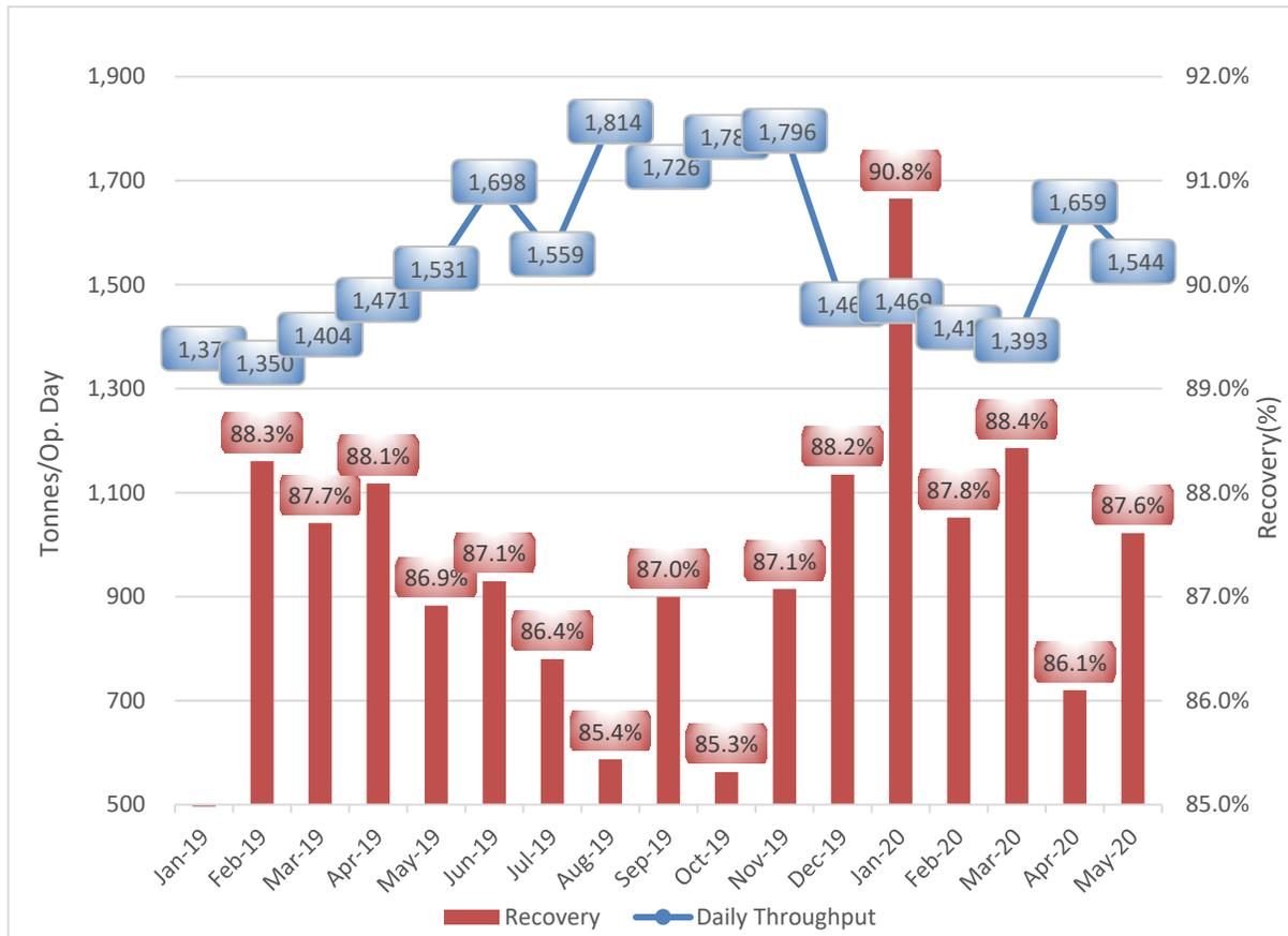
The plant capacity is more than current or planned production. Production is not plant constrained. The plant produced 40,682 ounces of gold at a recovery of 86.94% for 2019. For 2020 YTD, gold production was 20,690 ounces at a recovery of 88.06%.
