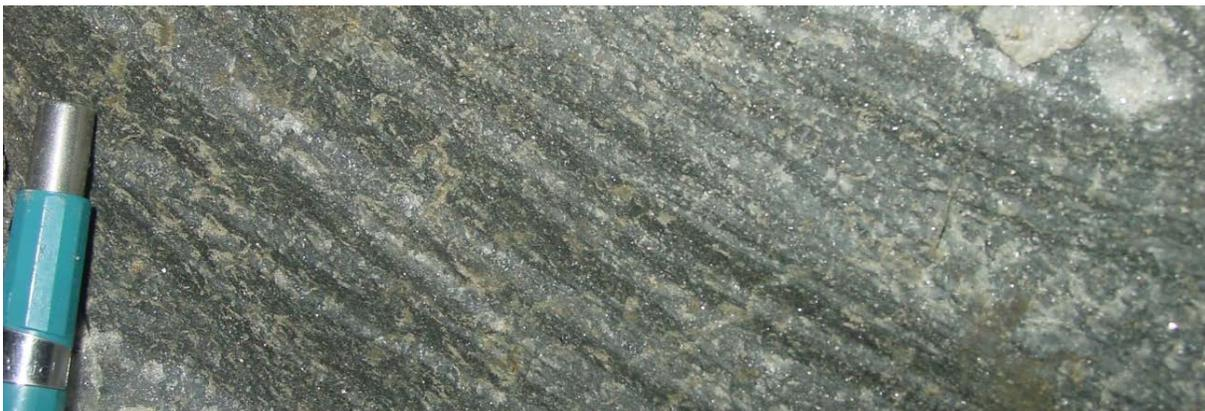
**FIGURE 7-10 PENETRATIVE EXTENSIONAL CLEAVAGE IN COMPETENT ROCKS, PILAR MINE**
