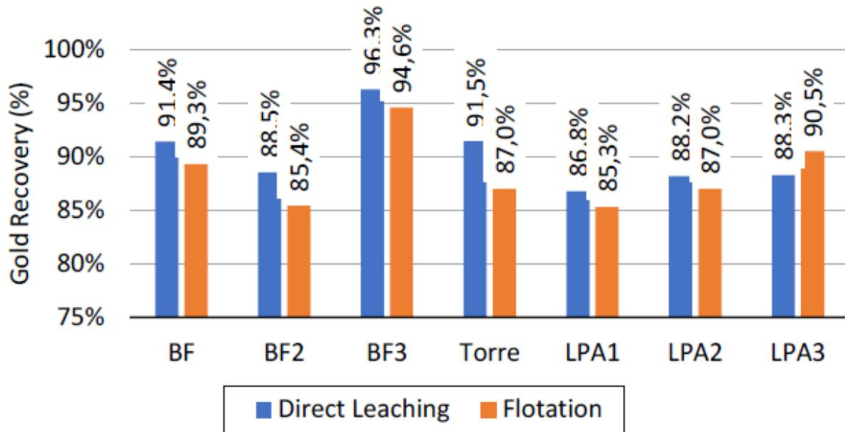
The graph above shows that there is a good correlation between direct leaching tests and flotation test results (gravimetric concentration + flotation + concentrate leaching). Further test work requiring more sampling may be warranted to confirm the correlation.
