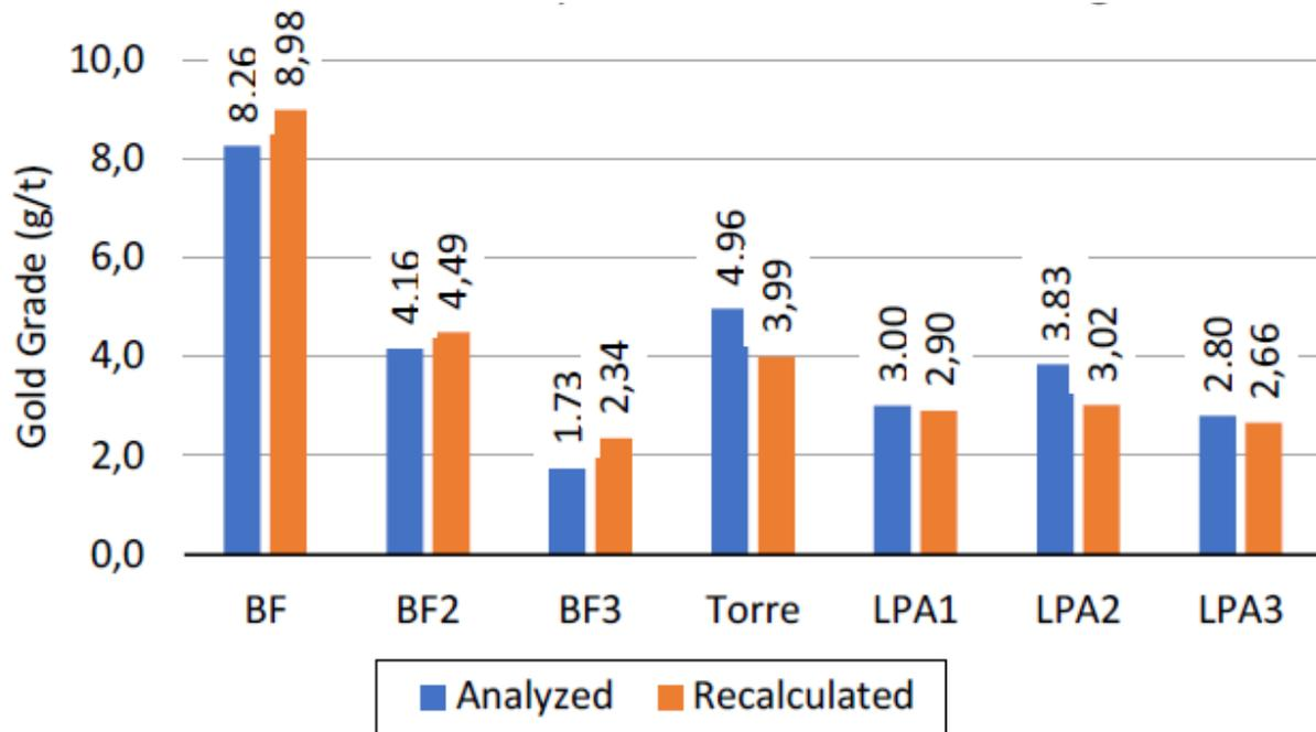
The averages of all the results of the gravimetric concentration tests, performed prior to the leaching and flotation tests showed similar results, independent of the grind. The results are shown below, in Figure 13-3.
