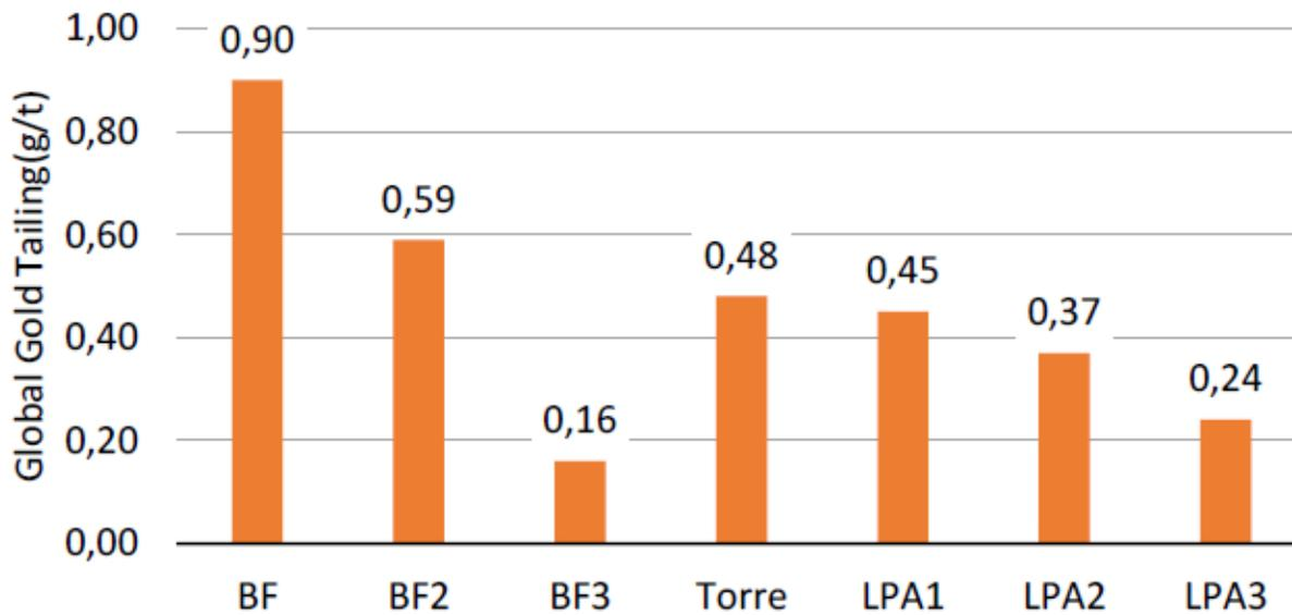
Figure 13-12 shows the comparison of overall recoveries of flotation tests with the overall recoveries of leaching tests, at a P<sub>80</sub> grind of 75 µm.
