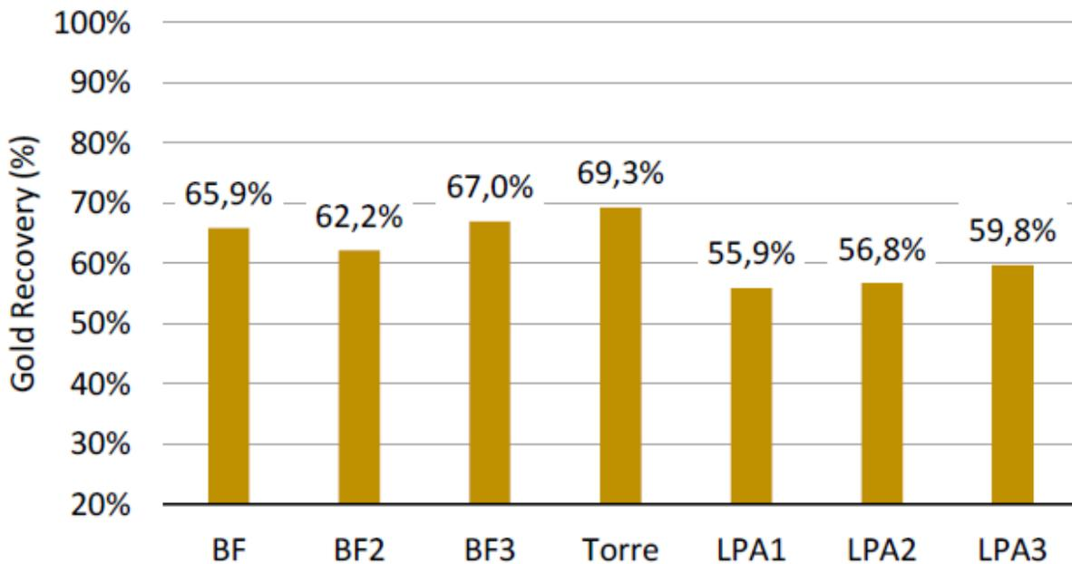
The high recoveries of free gold can justify the variation in the assayed versus calculated head gold content of the various tests performed shown earlier in Figure 13-2.
