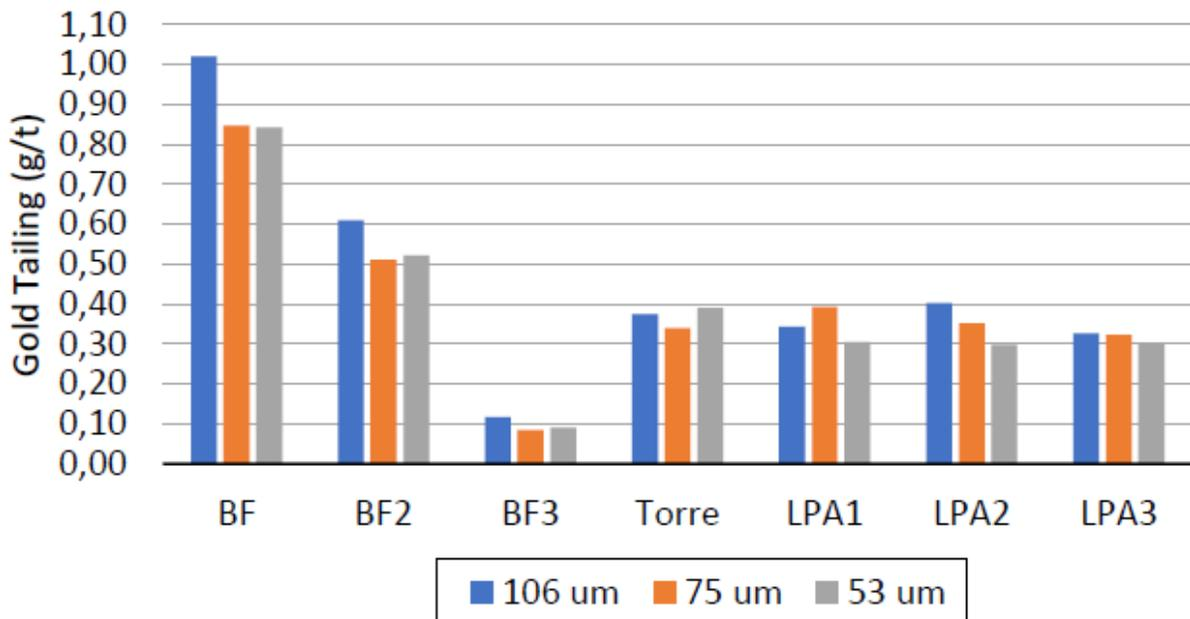
The results show that grinding equal to or below  $P_{80} = 75 \mu\text{m}$  reduces tailings values. The final recovery is naturally influenced by the head content of the tests, showing that the assessment of the contents of the tailings is important.
