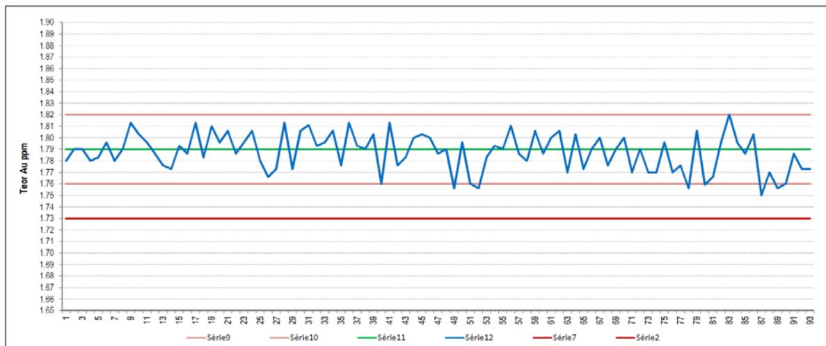
**FIGURE 11-3 CONTROL CHART FOR EXTERNAL CHECK SAMPLES, 2018 - JAGUAR VS. ALS CHEMEX**
